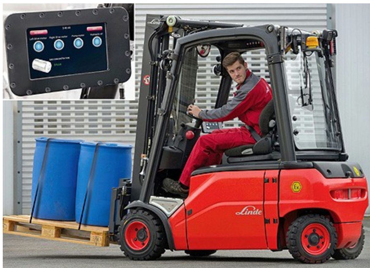
The innovative, radio-controlled gas warning system from French specialists Centrexpert is now available as an option for Linde electric forklift trucks used in explosion-protection zone 2 with a load capacity of between 1.4 and 3.5 tonnes.
