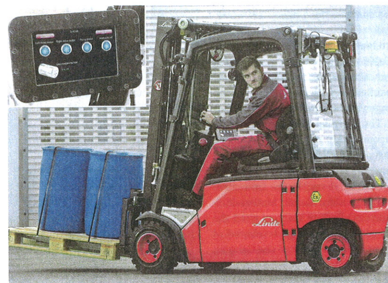
The radio-controlled gas warning system from French specialists Centrexpert is available as an option for Linde electric forklift trucks used in explosion-protection zone 2 with a load capacity of between 1.4 and 3.5 tons.
